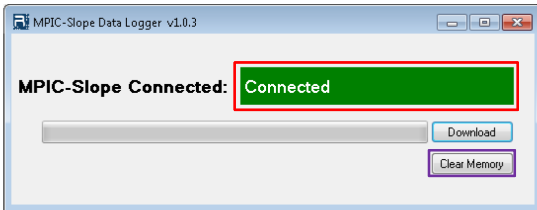
FIGURE 5.4: MAKE SURE THE LABEL INSIDE THE RED RECTANGLE IS GREEN AND SAYS "CONNECTED" AND PRESS THE "CLEAR MEMORY" BUTTON INSIDE THE PURPLE RECTANGLE.
