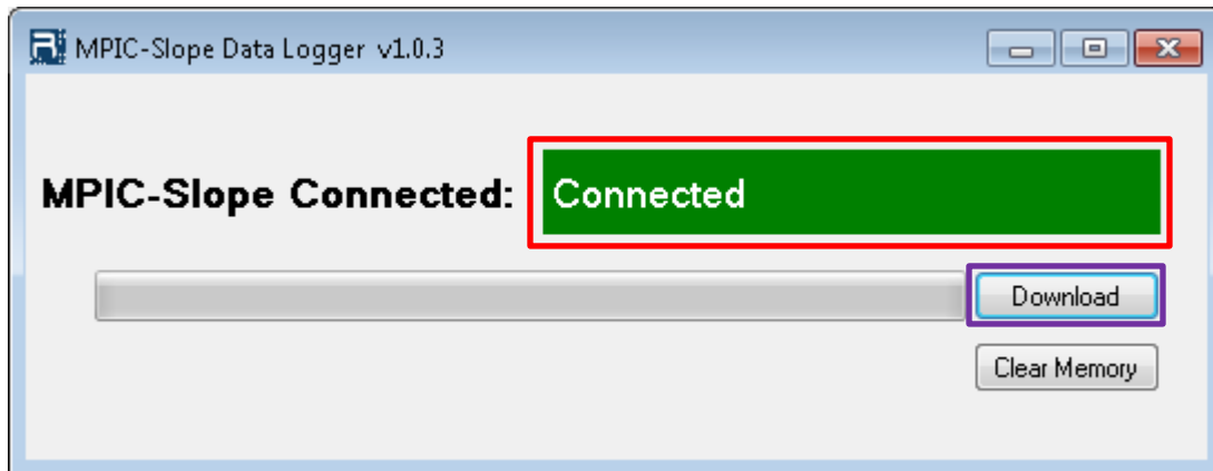
FIGURE 5.3: MAKE SURE THE LABEL INSIDE THE RED RECTANGLE IS GREEN AND DISPLAYS “CONNECTED” AND PRESS THE “DOWNLOAD” BUTTON INSIDE THE PURPLE RECTANGLE.
