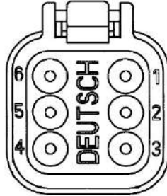
FIGURE 4.1: THE MPIC-SLOPE CONNECTOR (PART NUMBER: DT06-6S)
