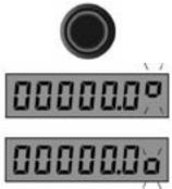
The last digit on the right blinks up and down indicating the hour-meter function. The hour-meter cannot be reset.
