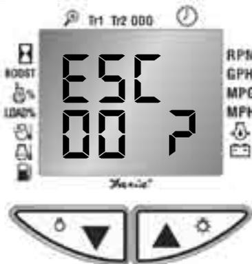
Step 2. *Push and Hold the Up and Down buttons together* until you exit the service mode.
