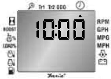
Step 2. Push and hold the MODE button until the display clock is reset to zero.
