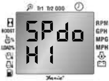
Faria Serial Bus Speedometer Lower limit value setup menu:
