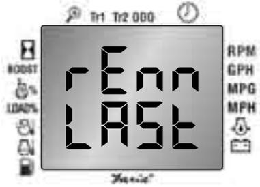
Step 5. Push and hold the UP and DOWN buttons together until the screen returns to the Start Menu.
