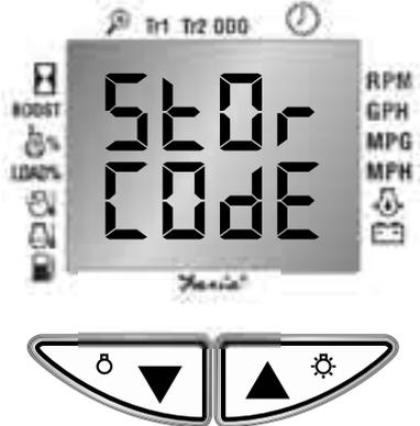
Step 3. Press and Hold the UP and DOWN buttons together until the CAN Info Center™ beeps (a long beep). The CAN Info Center™ may display a wait message.
