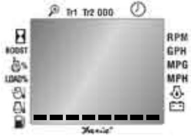
One Segment lit and flashing, the Fuel tank is empty. Eight segments lit, the tank is full.
