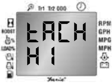
Faria Serial Bus Tachometer Lower limit value setup menu:
