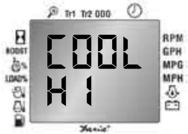
Faria Serial Bus Coolant Temperature gauge Lower limit value setup menu:
