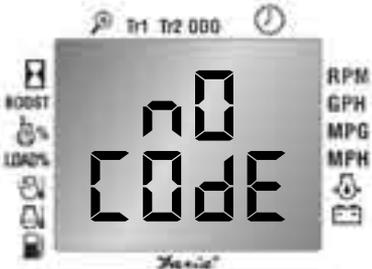
If the engine ECM does not support the DM2 delete using the J1939 protocol, the CAN Info Center™ will display:
