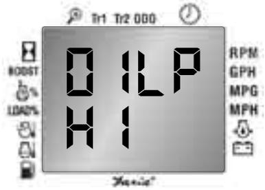
Faria Serial Bus Engine Oil pressure gauge Lower limit value setup menu:
