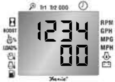
(1234) and (000) are the data which represent the engine configuration information sent from the Engine ECM via the CAN Data Bus.
