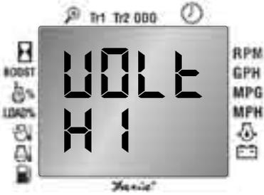
Faria Serial Bus Voltmeter Lower limit value setup menu:
