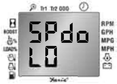
Step 3: Push and Hold both the UP and the DOWN buttons together until the display changes:
