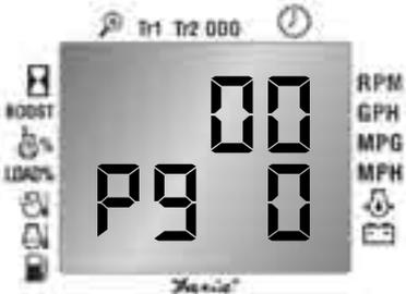
Step 7: Push and Hold both the UP and DOWN buttons together until the screen changes to:
