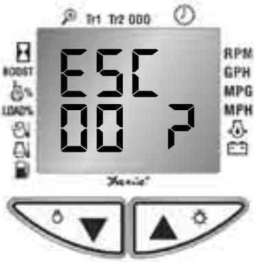
Step 2. **Push and Hold the Up and Down** buttons together to exit the service mode.
