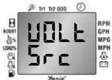
Step 3: Push and Hold both UP and DOWN buttons until the display changes:
