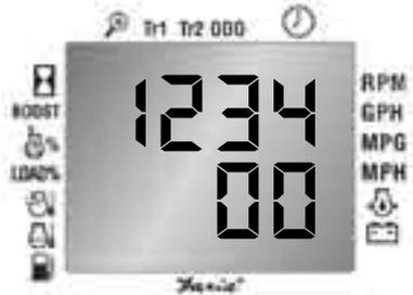
The upper display (1234) is the Suspect Parameter Number (SPN). The value can change from 0-9999 according to the codes from the engine ECM.
