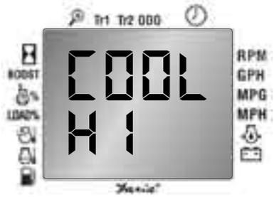
This will set the upper limit value of the Faria serial bus Coolant Temperature gauge.
