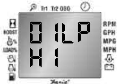
This will set the upper limit value of Faria serial bus engine Oil Pressure gauge.
