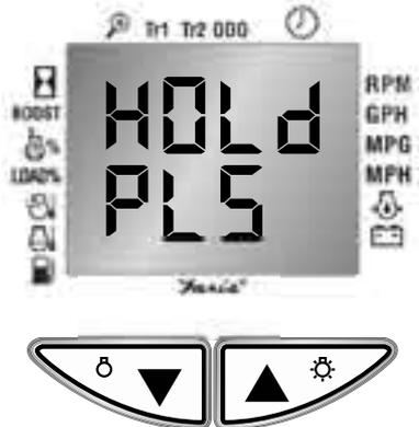
A “HOLD PLS” means the CAN Info Center™ is communicating with the engine ECM. Once all the information has been received, the display will switch to the information screen automatically.
