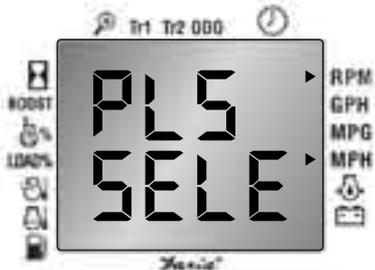
Step 9. Use the UP button to move the function indicator to select the desired default function for top display window. (the indicator moves only in a clockwise direction.)
