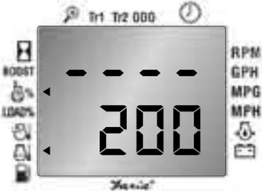
In this example the Accelerator Pedal Position shows not available and the Coolant Temperature shows 200 ° F.
