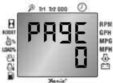
Step 4. Press and hold the MODE button until the CAN Info Center™ beeps (a long beep). This will reset all of the former calibration settings at all speed calibration points. The Speedometer calibration will be canceled.
