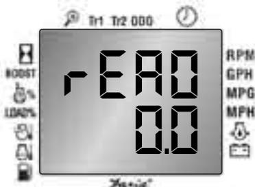
0.0 represents different values depending on whether the CAN Info Center™ has been calibrated. If Step 4 was executed correctly, the initial value should be 0.0.
