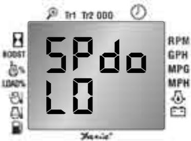
Faria Serial Bus Engine Oil pressure gauge Upper limit value setup menu:
