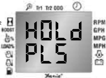
A “HOLD PLS” means the CAN Info Center™ is communicating with the engine ECM. No action is required. Once the desired information has been received from the engine ECM, the display will switch to the information screen automatically. (There may be times where the wait message will be too fast to be seen. This is normal.)
