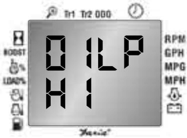
Step 3: Push and Hold both the UP and the DOWN buttons together until the display changes:
