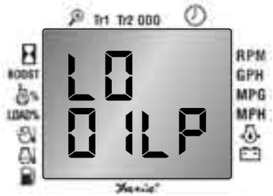
This will set the lower limit value of the Faria serial bus engine Oil Pressure gauge.
