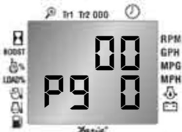
The Upper display shows the Warning Lamp Status in a decimal based numerical value (00). The value of (00) can be changed from 00-255 according to different codes received from the Engine ECM via the CAN Data Bus.
