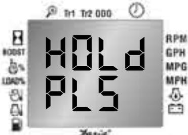
A "HOLD PLS" means the CAN Info Center™ is communicating with the engine ECM. No action is required. Once the desired information has been
