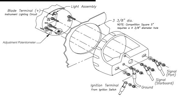
The Faria® Marine dual engine synchronizer is designed to indicate engine synchronization extremely accurately when the speeds of the two engines are compared to each other. Engine synchronization may be difficult at idle speeds. For proper operation, both engines must be of the same type, have the same number of cylinders, and have similar ignitions. Malfunctioning ignition systems or high speed "point bounce" will result in inability to sync properly.
